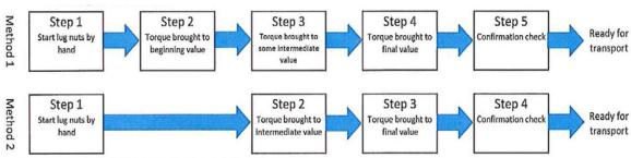
Figure 1. The two methods typically used in manufacturing and wheel assembly.
